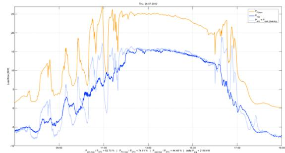
**Figure 4: Simulation of the power generated by the distributed PV fleet (orange), measured (dark blue) and calculated (light blue) cumulated power of the area on 26 July 2012. The congruence between the dark and the light blue curve indicates the accuracy of the simulation. Only one measurement station is used as simulation input. Simulation and real measured data match rather well for a clear sky.**
