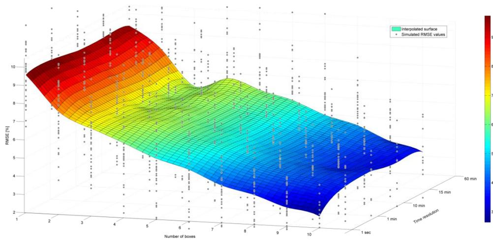
**Figure 9:** Three dimensional plot of the root mean square error as a function of the number of measurement stations on the x-axis and the time resolution on the y-axis. The grey points correspond to all simulated values and the surface is gained by interpolation.
