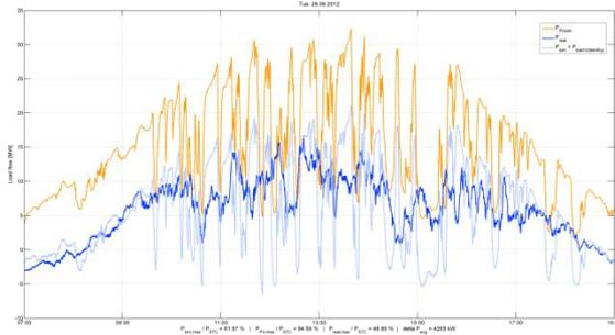
**Figure 5: Simulation of the power generated by the distributed PV fleet (orange), measured (dark blue) and calculated (light blue) cumulated power of the area on 26 June 2012. Only one station is used as simulation input.**
