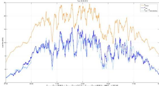
**Figure 6: Simulation of the power generated by the distributed PV fleet (orange), measured (dark blue) and calculated (light blue) cumulated power of the area on 26 June 2012. Ten stations are used as simulation input.**
