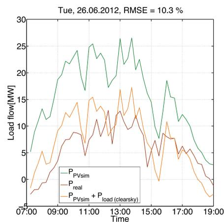
**Figure 2b:** Simulation based on just one measurement sensor. One sensor is not sufficient to model the spatial smoothing of the feed-in power of the distributed PV systems and hence the grid condition on a fluctuating day. The rmse is significantly high with 10.3 %.
