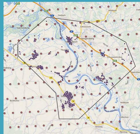
**Fig. 1b:** Investigation area and measurement points (red) covered by satellite. Data is recorded every 15 minutes in a spatial resolution of ca. 2.6 km<sup>2</sup>. PV systems in the area (blue) are assigned to the single pixels and each pixel is simulated separately with its measured data and the respective PV capacity as input.
