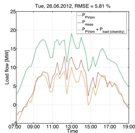
**Figure 2c:** Simulation on the basis of satellite data. Simulated and measured load flow match rather well. The rmse amounts to 5.81 %. Simulated power is slightly lower than the measured curve and the rather high smoothing effect is modeled well.
