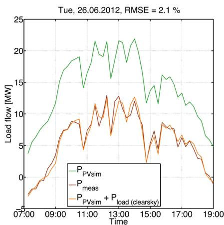
**Figure 2a:** Simulation on the basis of ten distributed measurement devices. In order to quantify simulation accuracy, the root mean squared error (rmse) is applied. Rmse is only 2.1 %. Spatial smoothing of the distributed PV fleet is modeled properly.
