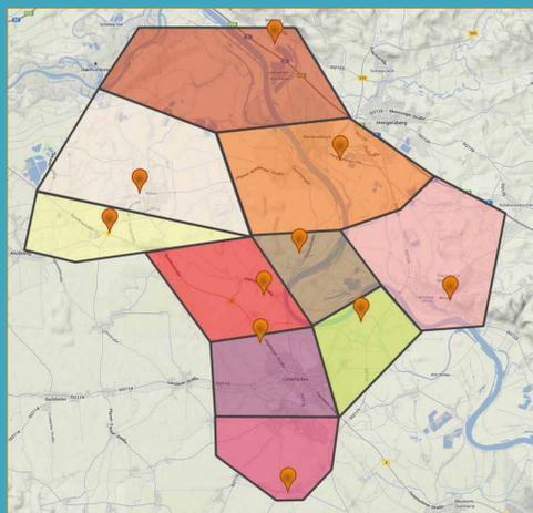
**Fig. 1a:** Investigation area with the distributed measurement system. Spatial resolution amounts to 10 km<sup>2</sup> and the measurement interval is 3 seconds. The area is subdivided into ten subareas and simulated separately using the corresponding device's data and the installed PV capacity.
