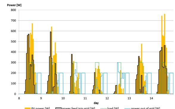
Fig. 6: Behavior of the power, fed into the grid, the load and the power out of the grid are shown for some days in July in Nuremberg.
