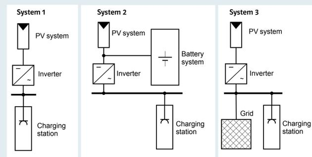
Fig. 1: Three types of systems have been investigated - the standalone system (left), the system with a buffer battery (middle) and the system with grid connection (right).
