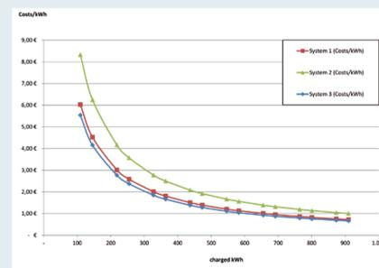
Fig. 8: Comparison of the electricity production costs of all three systems, depending on the number of charged kWh.
