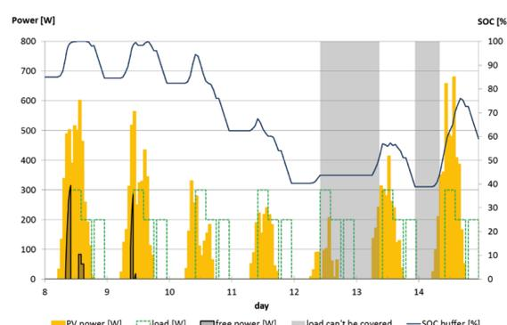
Fig. 4: Behavior of the load, the SOC and the time, the load cannot be satisfied are shown for some days in July in Nuremberg.
