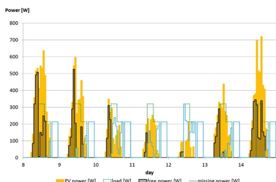
Fig. 2: Behavior of the load and the missing power are shown for some days in July in Nuremberg.
