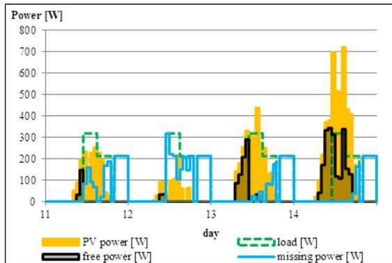
Figure 3: System 1 – power behavior over four days.
