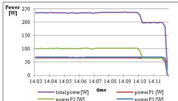
Figure 9: Real system – power values during the charge of an e-bike.
