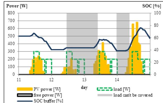
Figure 5: System 2 – power behavior over four days.
