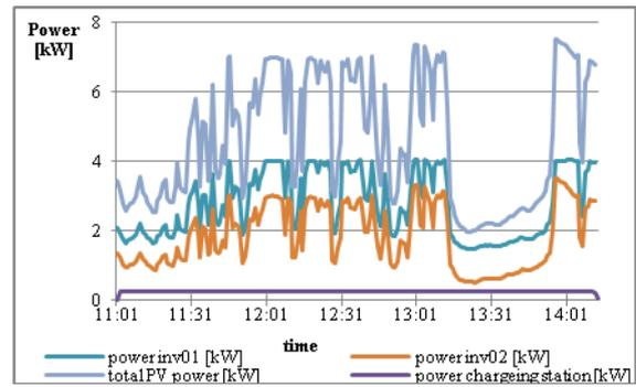
Figure 10: Real system - power values in Sengenthal during charging an e-bike.
