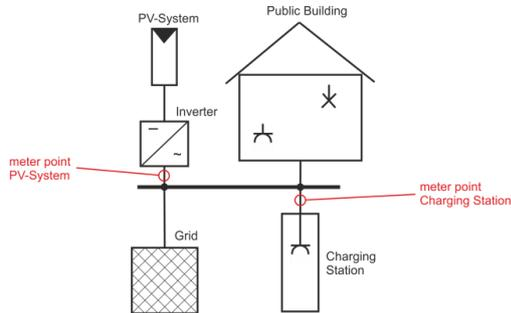
Figure 8: Basic structure of the real system. The inverter consists of two sub inverters.
