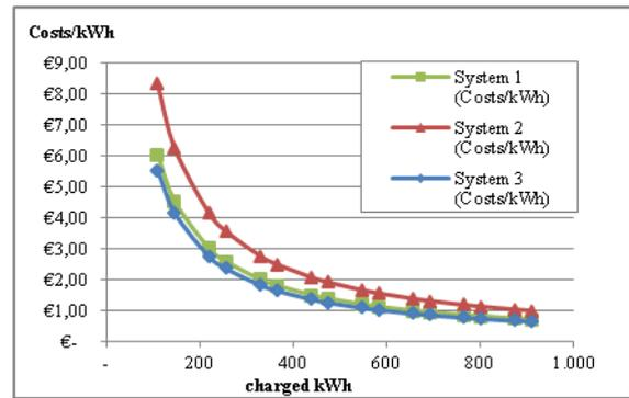
Figure 15: Comparison of the electricity production costs of all three systems, depending on the charged energy.
